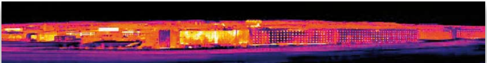
Panorama image taken with 200x150 pixel resolution and <70mK thermal sensitivity.
