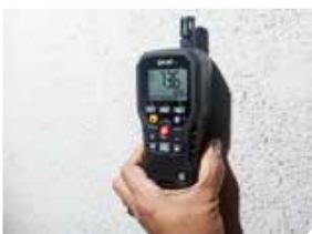
Quickly assess upto 0.75 inches deep in Internal Pinless moisture mode
